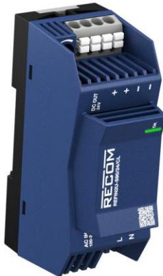
The REFIN2U-S90/24/CL is presented in the popular 'step-shape' DIN rail format and is just 36mm in width, weighing in at only 151g. Extending mounting flanges allow the part to be panel-mounted if wished, and particular attention has been paid to eliminating acoustical noise – an important consideration in office or domestic installations.
